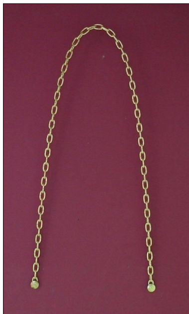
Fig. 3. Inversion of Fig. 2 shows the theoretical 'catenary arch'.
