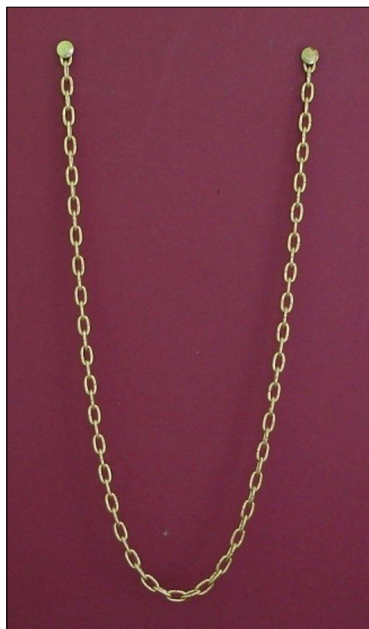
Fig. 2. A chain hanging freely in equilibrium displays a catenary curve.
